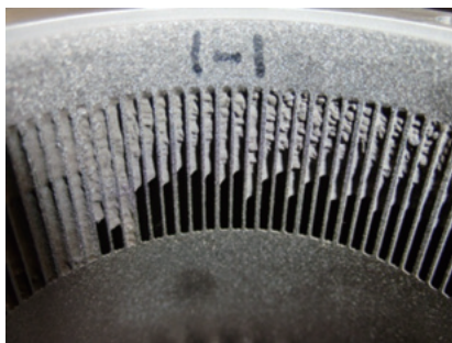
Fig. 15 Congealed powder remaining after machining work to remove reinforcing ring
