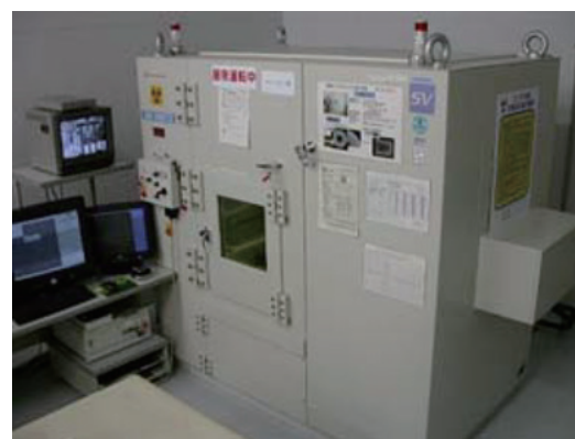
Fig. 23 Shimadzu Micro-focus X-ray CT System (SMX-225CT-SV3)
