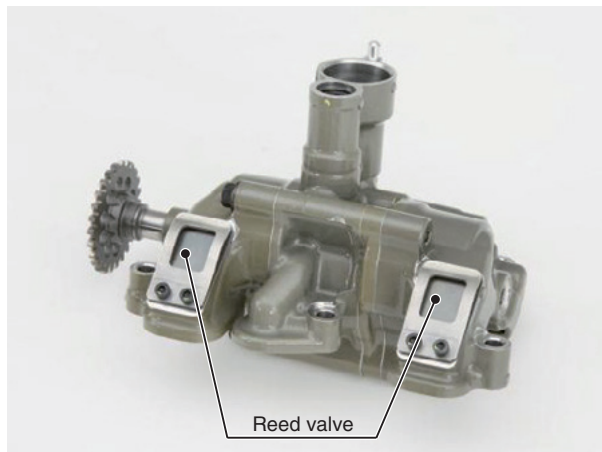
Fig. 9 External view of oil pump assembly
