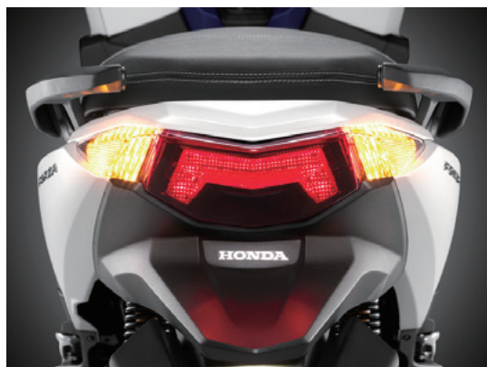
Fig. 20 LED tail and brake light
