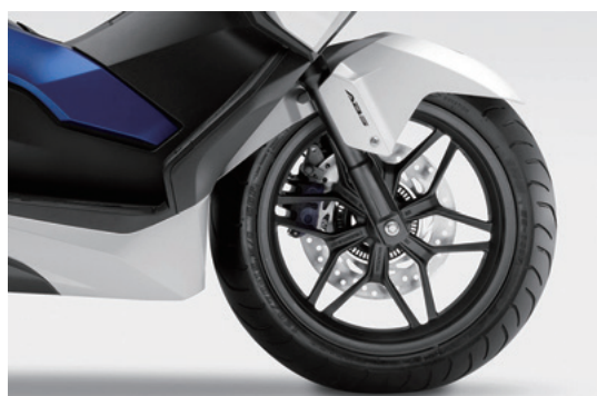
Fig. 18 Front wheel and front fork with bottom case
