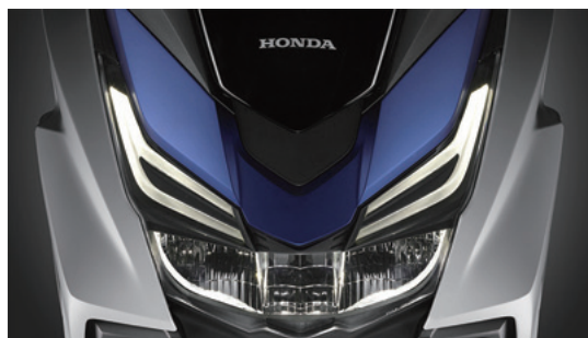
Fig. 19 Dual LED head lights and LED position lights
