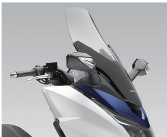
Fig. 17 Side mirrors installed with turn signal lights
