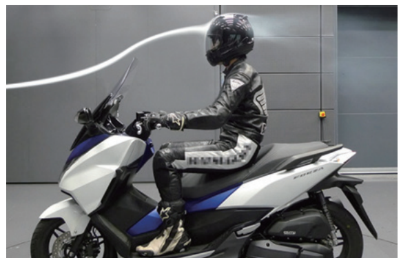
Fig. 15 Design verification using wind tunnel
