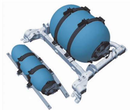
Fig. 12 Image of H 2 tank installation
