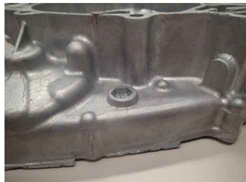
Fig. 26 Raw material appearance after 10000 shots
