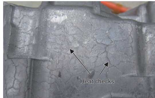
Fig. 16 Transferred heat checks
