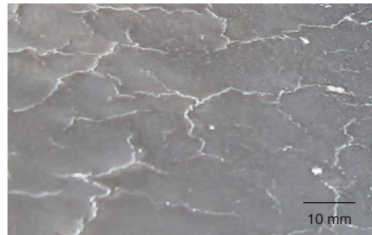
Fig. 17 Heat checks occurred on die surface
