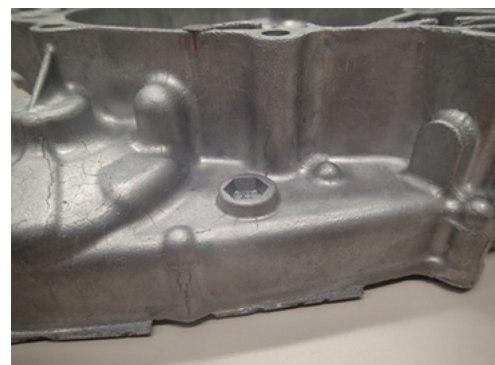
Fig. 26 Raw material appearance after 10000 shots
