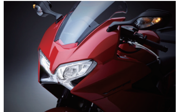
Fig. 9 Image representation using LED light guiding panel in the VFR800F, 2014 year model
