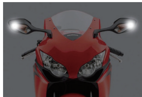
Fig. 4 Front position lights (at rear view mirror) in the CBR1000RR, 2008 year model
