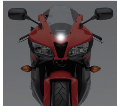
Fig. 3 Front position light (at center) in the CBR600RR, 2007 year model
