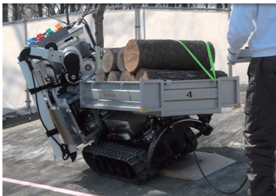
Fig. 16 Traveling on slope using overturn suppression
