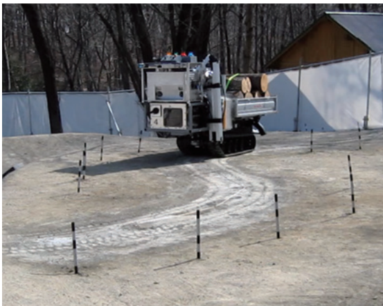
Fig. 9 Automatic traveling by electromagnetic navigation
