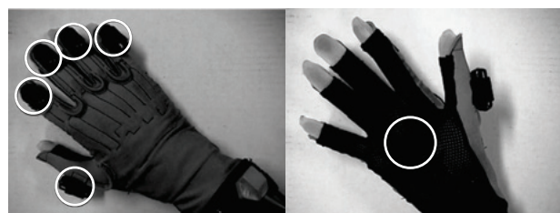
Fig. 1 Vibrators on right-hand glove. Five small motors are placed at circled locations on the tops of the fingers and one on the palm.
