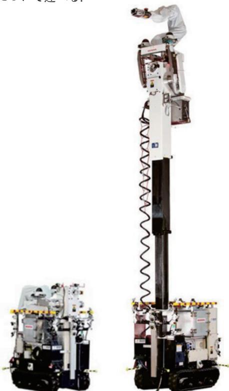
Fig. 1 High-Aaccess Survey Robot The driving posture (left) and higher posture (right)
