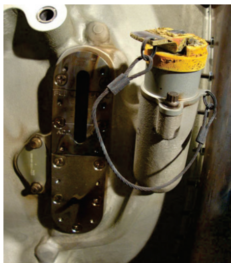
Fig. 2 Fire exposure area of oil tank after test
