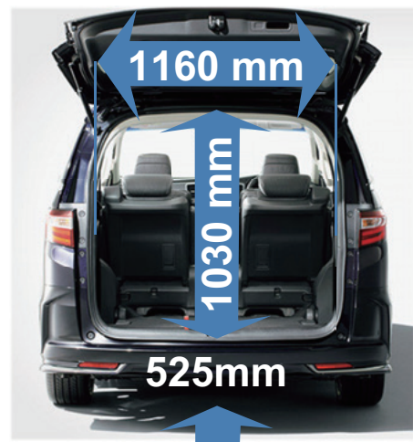
Fig. 16 Dimensions of tail gate opening
