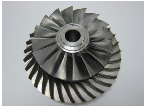
Fig. 12 High-flow centrifugal impeller of small-scale rig
