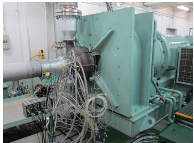
Fig. 13 Small-scale rig of centrifugal compressor
