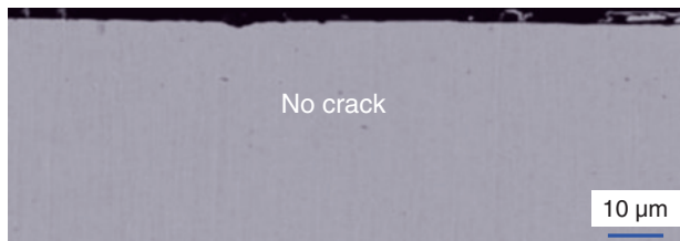
Fig. 15 Sectional view of pulley surface
