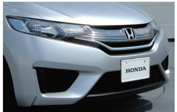
Fig. 9 Layered wing bumper
