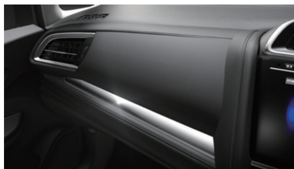
Fig. 22 Soft pad panel
