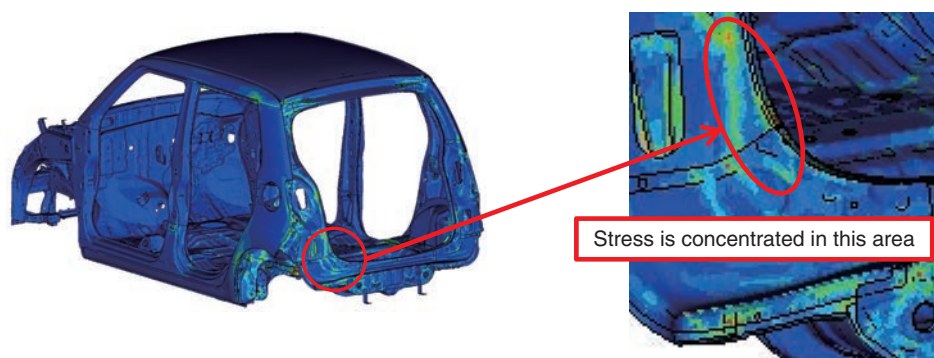
Fig. 14 Result of stress analysis by torsion test
