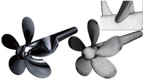
Fig. 4 Propeller CAD model (left) and computational mesh (right)
