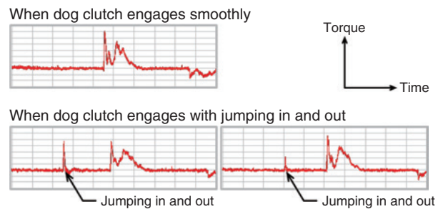
Fig. 16 Time history of torque when dog clutch engages
