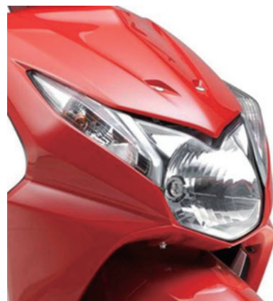
Fig. 6 Integrated headlight unit with turn signals
