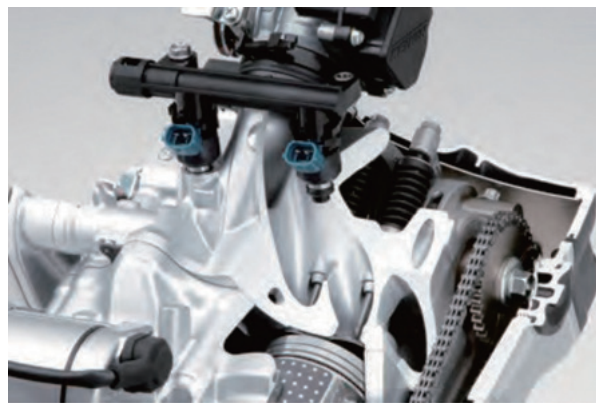
Fig. 9 Branched intake port
