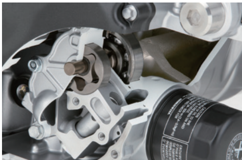
Fig. 12 Oil pump driven via balancer shaft
