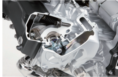
Fig. 13 Water pump driven via camshaft
