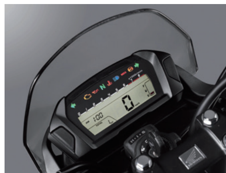
Fig. 14 Meter display unit of NC700S
