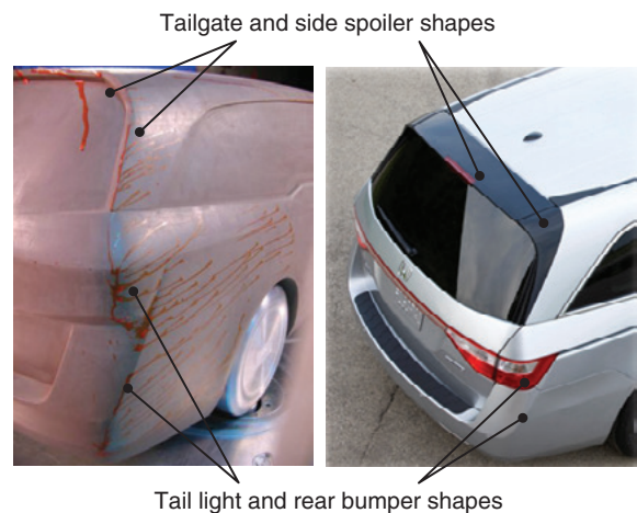
Fig. 13 Wind tunnel development of rear flow separation
