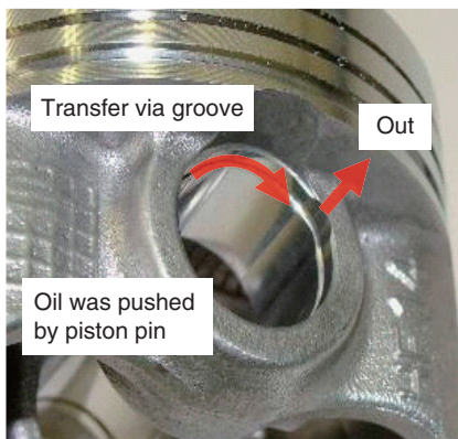
Fig. 9 Oil transfer path in piston pin hole
