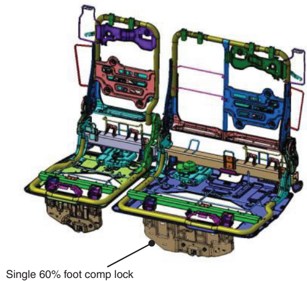
Fig. 21 2011 Odyssey 3 rd row seat structure and 60% foot comp single lock
