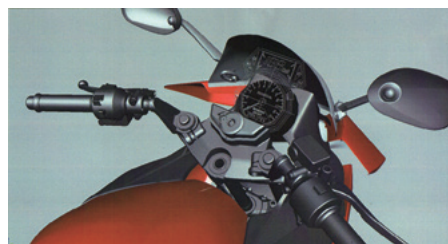
Fig. 5 3D model: Gauges and switches
