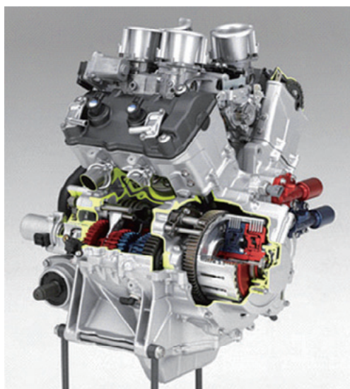
Fig. 2 External view of V4 engine with newly developed dual clutch transmission
