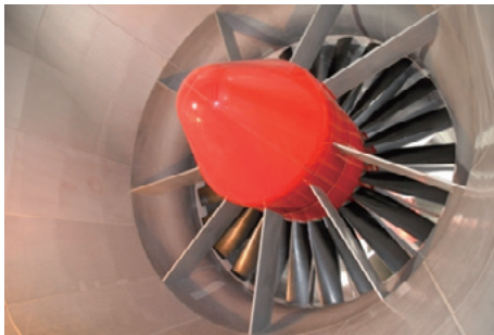
Fig. 5 Main fan with 9 inlet guide vanes, 24 rotor blades and 35 stators
