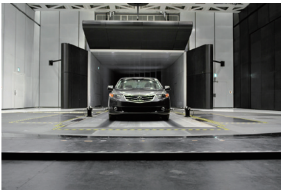
Fig. 2 Open jet test section view from upstream with collector in background
