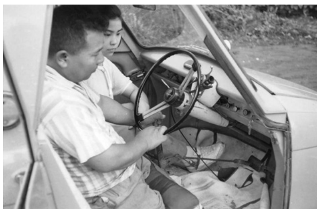
Fig. 1 Manually operated auxiliary driving device
