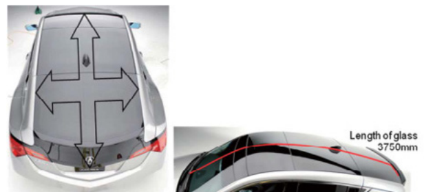
Fig. 11 Long and wide expanse of glass of ZDX panoramic roof
