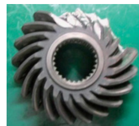
Fig. 16 Status of gear damaged in durability test
