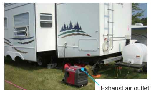
Fig. 2 Example of use as camper power source
