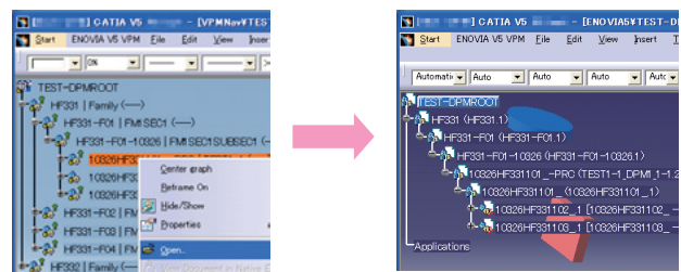
Fig. 6 Operation to access 3D data from structure tree
