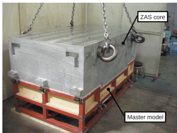
Fig. 12 Combination of master model and ZAS core
