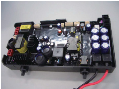
Fig. 11 DC-DC converter unit
