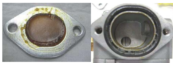
Fig. 15 Residue that drained into cup (use for 50 hours)
