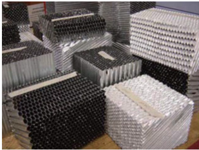
Fig. 4 Samples cut from honeycomb block at different angles
