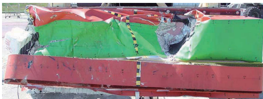
Fig. 1 Typical damage to honeycomb barrier seen after FMVSS 301 high speed rear crash test
