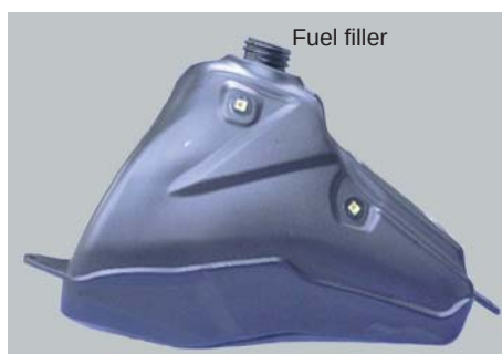
Fig. 1 Appearance of saddle-type fuel tank for motorcycle
