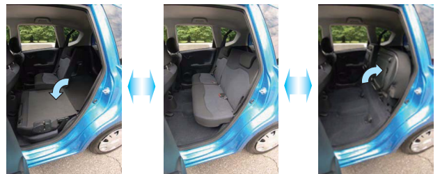
Fig. 11 One motion dive-down
