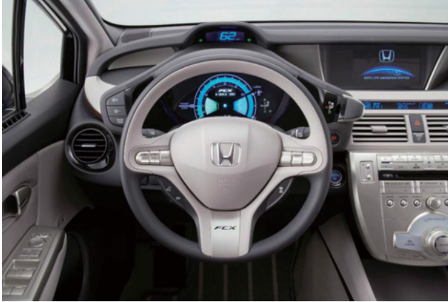
Fig. 2 FCX multiplex meters(multi-layered instrument panel)
