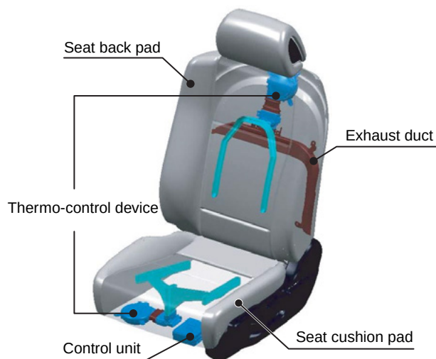
Fig. 2 Heated and cooled seat
