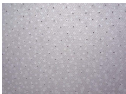
Fig. 11 Seat covering material (Honda bio-fabric)
