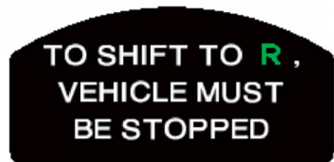
Fig. 12 R inhibitor in operation
