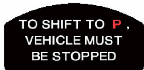
Fig. 13 P inhibitor in operation
