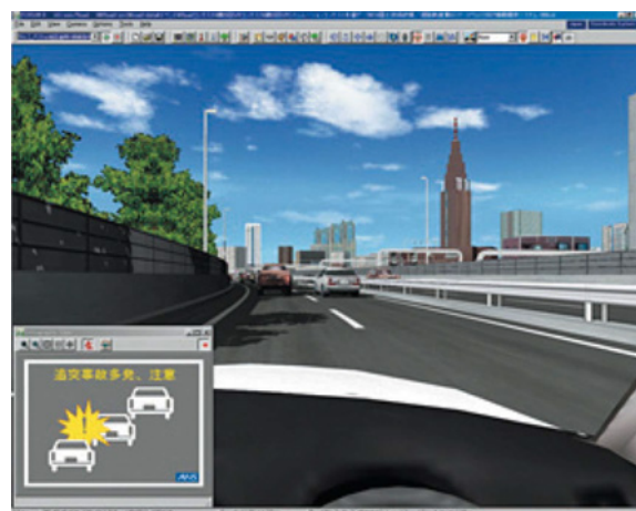
Fig. 9 Providing information with digital road map data
