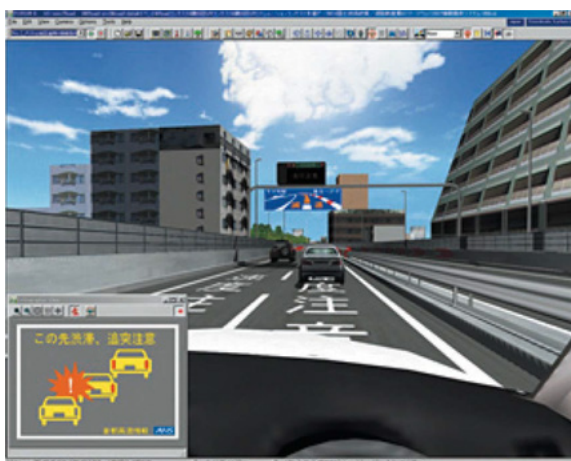
Fig. 6 Providing information on obstacles ahead
