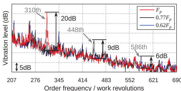
(b) Spectra of transmission case vibration occurring when changing feed pitch of grinding wheel
