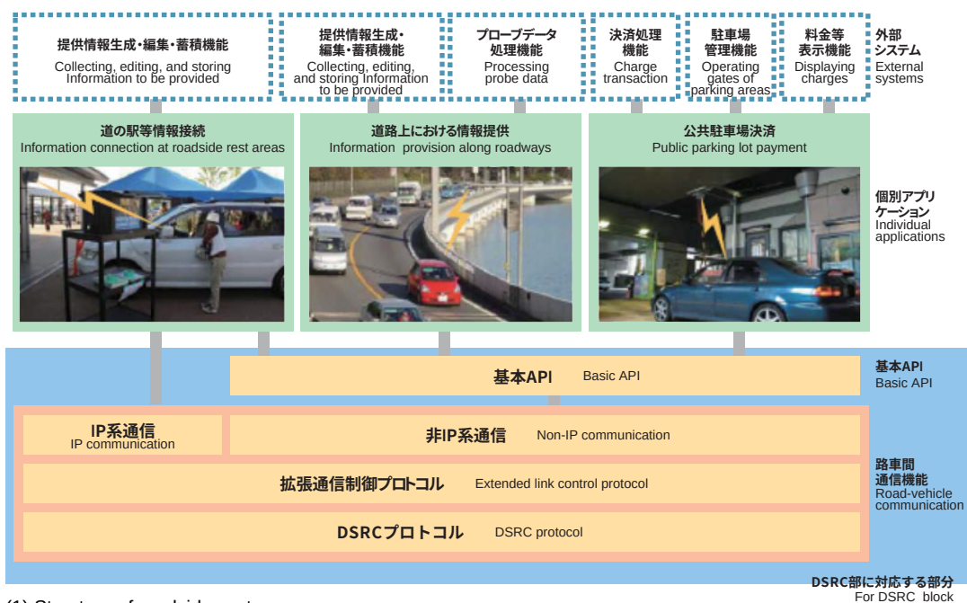
(1) Structure of roadside system
