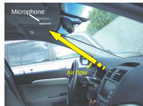
Fig. 5 Direct airflow from air conditioner
