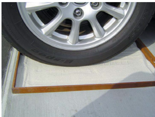
Fig. 7 Measuring resistance through tires with sand between tire and concrete pad
