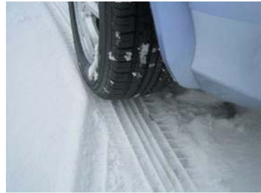
Fig. 8 Measuring resistance through tires with snow between tire and concrete pad
