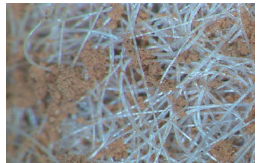
Fig. 3 Dust (1-50 \mu\text{m} ) and other substances trapped in filter-fiber
