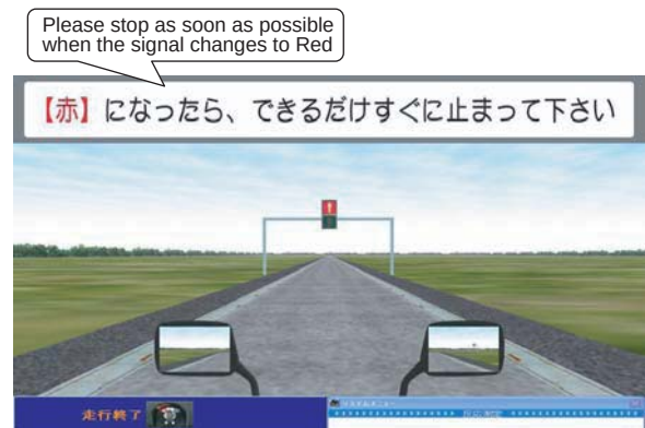
Fig. 12 Measuring delay in reaction movement
