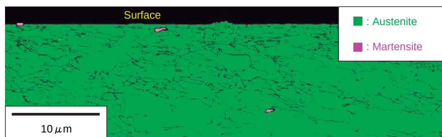
Fig. 11 Phase identification in surface structure after final annealing by EBSD analysis
