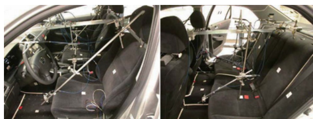
Fig. 6 Definition of microphone setup
