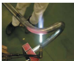
Fig. 10 Manual bending by specialist
