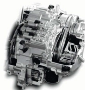
Fig. 1 CVT with torque converter
