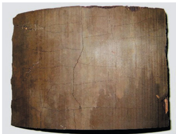
Fig. 3 Surface crack after 830°C x 300Hr aging
