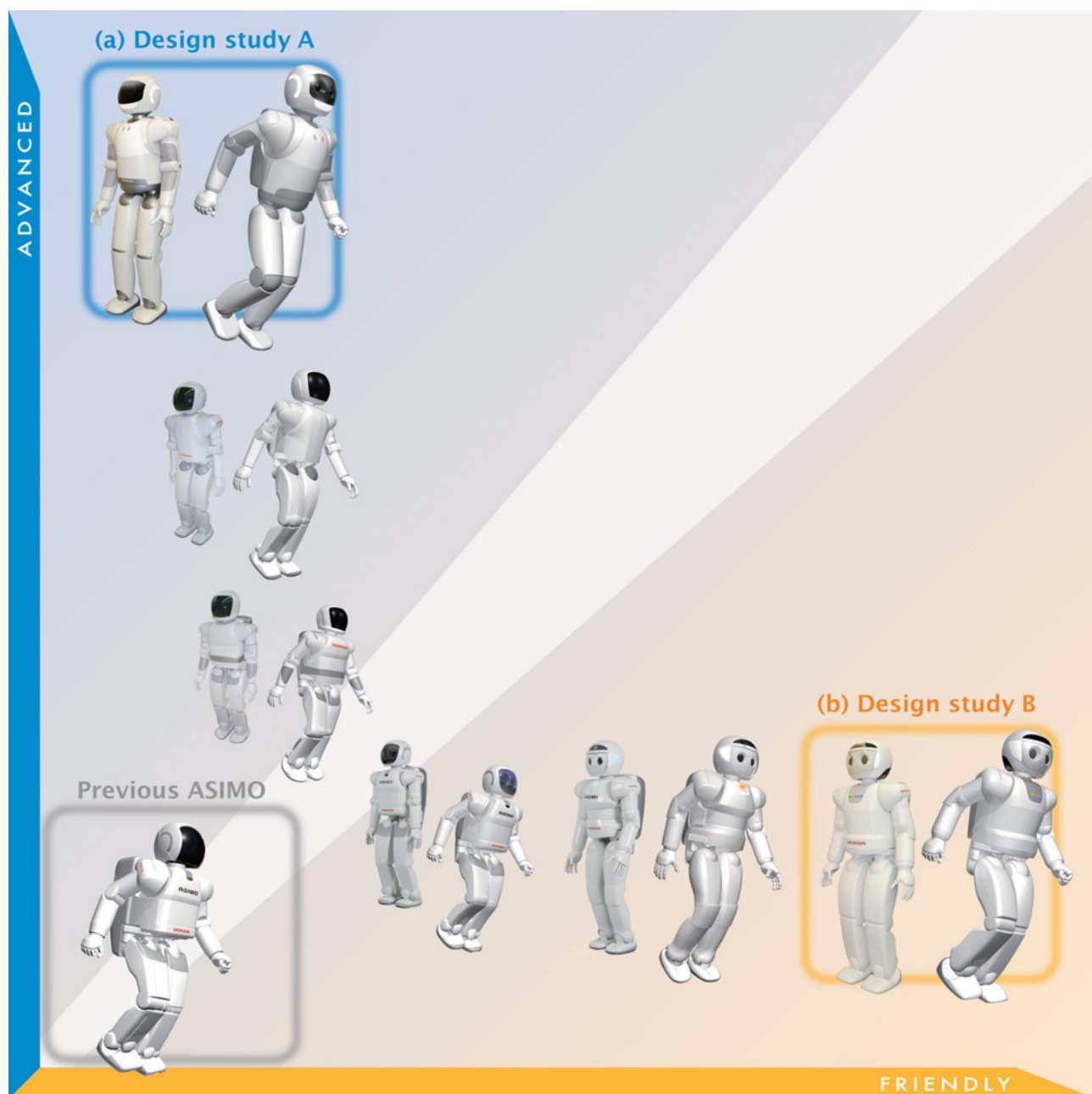
Fig. 3 Relation of design studies with previous ASIMO [(a) : advanced design, (b) : friendly design]
