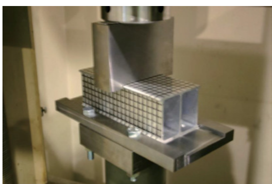
Fig. 9 Photograph of crush test device
