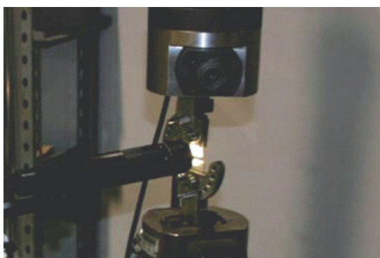
Fig. 8 Photograph of mixed-mode fracture test device
